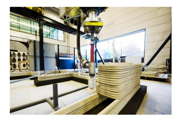
A print head of the 3-D concrete printer and some first samples of printed building elements. Credit: Rien Meulman
