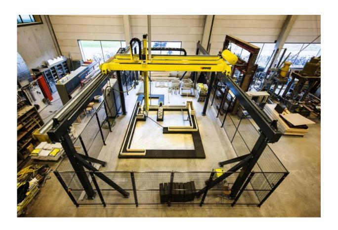
A top view of the concrete printer in the laboratory of the department Built Environment of Eindhoven University of Technology. Credit: Rien Meulman
