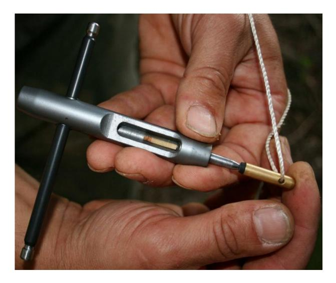
Fig. 3. Microcores of 2 mm in diameter and 1.5 cm in length (as the one visible here in the extracting chamber of the tool used) are collected using a very small borer. The sampling can thus be repeated on the same tree during the growing season to monitor wood formation with a high temporal resolution. Credit: Photo: Henri Cuny, WSL
