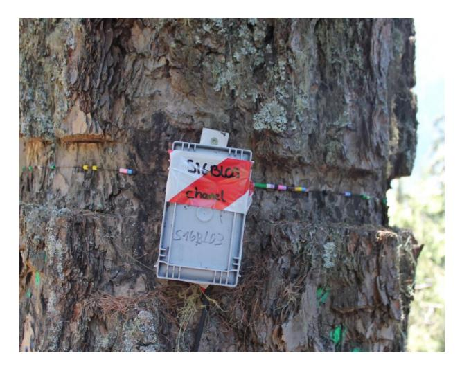
Fig. 2. Automatic dendrometers such as this one installed on a European larch in the Lötschental automatically measure and record stem circumference every 30 minutes, thus allowing scientists to monitor the dynamics of stem-girth variations. Credit: Henri Cuny, WSL
