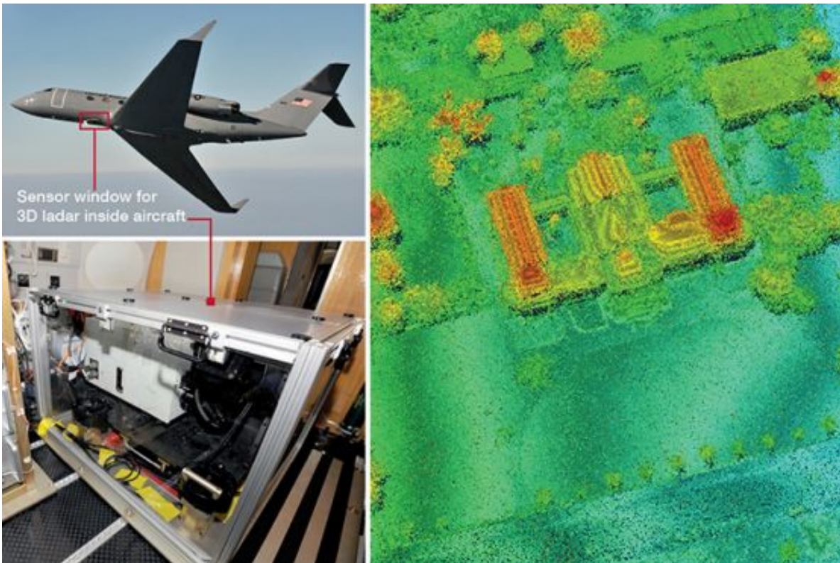
The Lincoln Laboratory-developed Airborne Ladar Imaging Research Testbed (ALIRT, at left) employs innovative Geiger-mode avalanche photodiode arrays
