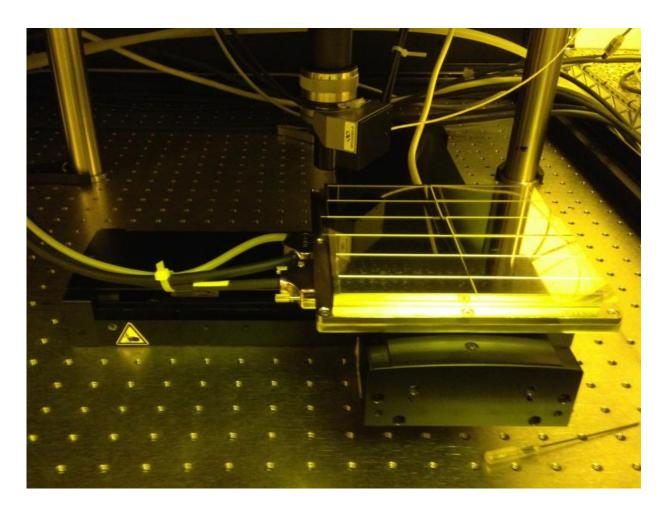
To understand how the direct-write laser scanner (DWLS) works, you have to understand that it doesn't have an inkjet--it prints light, and it prints in four dimensions. The DWLS has a moveable X-Y translation platform, on which substrates are placed, and the vertical final lens assembly through which the laser beam is focused to a tight spot. Credit: Michael Escuti, North Carolina State University
