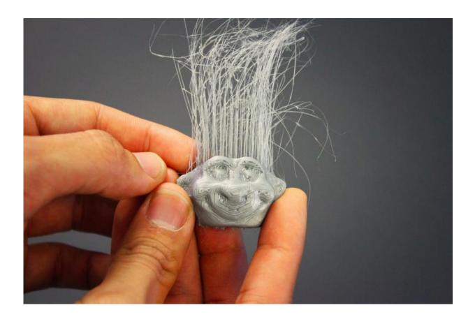
Researchers at Carnegie Mellon University have invented a way to produce hairlike strands, fibers and bristles using a common, low-cost 3-D printer. Credit: Carnegie Mellon University
