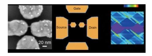
Left to right: a scanning electrode microscopy shot of the series of double-dot single-electron transistor (bright spots correspond to the cores of the gold nanoparticles); a schematic of the device; an experimental stability diagram. Credit: Majima/Tokyo Institute of Technology
