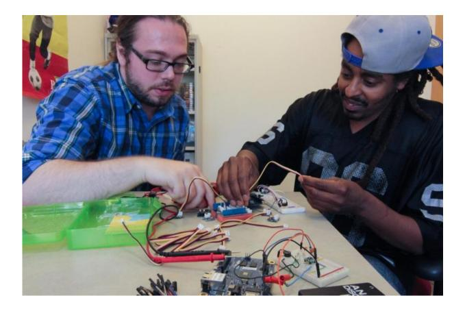
UCSD bioengineering master's student Michael Bajema and Ph.D candidate Amr Haj-Omar build a sensing device powered by an Intel Galileo prototyping compute board.
