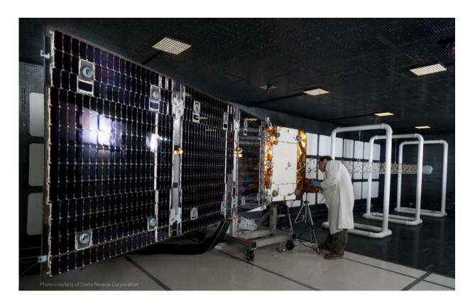
An ORBCOMM OG-2 satellite undergoes testing prior to launch. Credit: Sierra Nevada Corp
