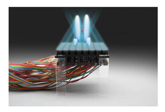
Holograms are tridimensional light-fields that can be projected from a two-dimensional surface. We have created acoustic holograms with shapes such as tweezers, twisters and cages that exert forces on particles to levitate and manipulate them. Credit: Image courtesy of Asier Marzo, Bruce Drinkwater and Sriram Subramanian, copyright © 2015.
