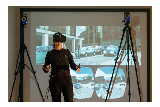
The pedestrian simulator can be connected with to other traffic-simulators. Credit: Uli Benz / TUM
