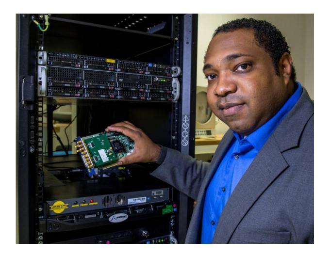
Philip Baldwin holds the custom-designed high-speed interface card that enables data transfer from Antarctica to White Sands, New Mexico, at about 300 Mbps. The electronics rack in the background is similar to the one inside the radome housing the new equipment. Credit: NASA/W. Hrybyk
