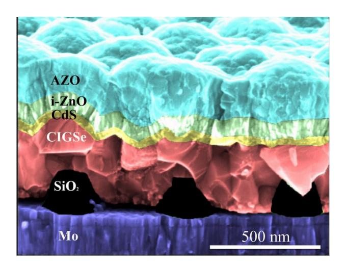
The SiO2 nanoparticles (black) have been imprinted directly on the molybdenum substrate (purple) which corresponds to the back contact of the solar cell. On top of this structured substrate the ultrathin CIGSe layer (red) was grown at HZB, and subsequently all the other layers and contacts needed for the solar cell. Since all layers are extremely thin, even the top layer is showing deformations according to the pattern of the nanoparticles. Credit: G.Yin / HZB
