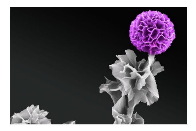
In full bloom: A scanning electron microscopy image produced by Jessica Wang of a vertical tetraanaline semiconductor crystal. Credit: Jessica Wang
