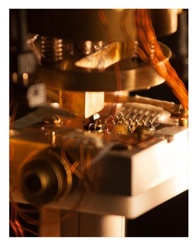
This microwave impedance microscopy (MIM) instrument was used to image
