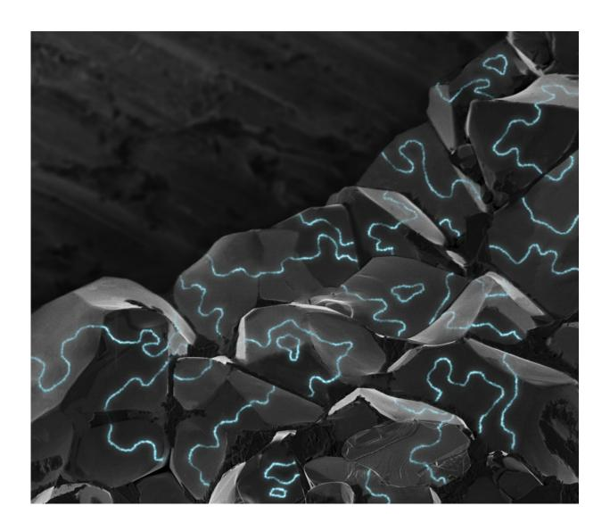
An illustration of electrically conductive areas (blue) along the boundaries of tiny magnetic regions, or domains, in chunky grains of a material that normally doesn't conduct electricity. This type of conductivity was postulated decades ago
