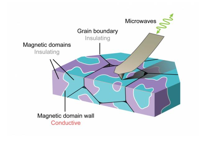
Scientists were able to make direct images of electrically conductive boundaries between a material's magnetic regions, or domains, using a technique called microwave impedance microscopy (MIM). The device sends microwaves down through the tip of a probe that is in direct contact with the material, and collects the microwave signals that are reflected back. Credit: Eric Yue Ma/Stanford University
