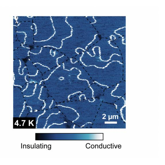
This image of a magnetic material taken with MIM shows that the bulk of the material is electrically insulating (dark blue regions) and the boundaries between magnetic domains are electrically conductive (white solid lines). Credit: E.Y. Ma et al., Science
