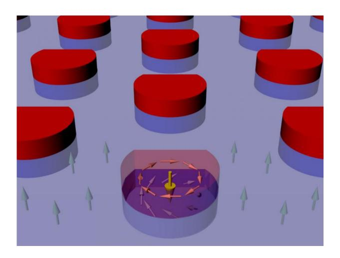
A magnetized cobalt disk (red) placed atop a thin cobalt-palladium film (light purple background) can be made to confer its own ringed configuration of magnetic moments (orange arrows) to the film below, creating a skyrmion in the film (purple arrows). The skyrmion, which is stable at room temperature, might be usable in computer memory systems. Credit: Dustin Gilbert / NIST
