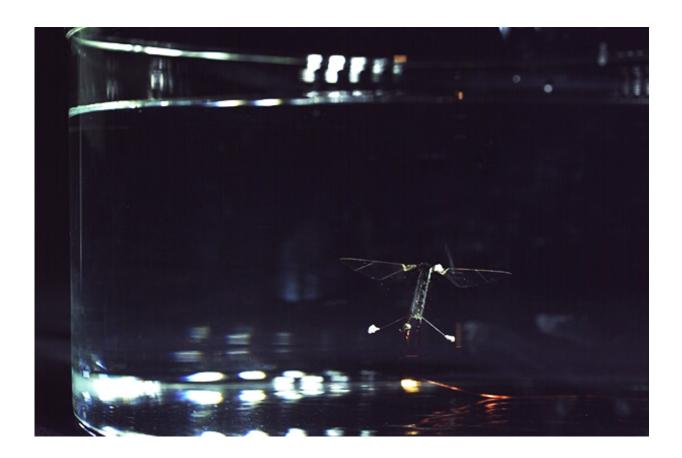
The Harvard RoboBee, designed in Wood's lab, is a microrobot, smaller than a paperclip, that flies and hovers like an insect, flapping its tiny, nearly invisible wings 120 times per second. Credit: Harvard Microrobotics Lab
