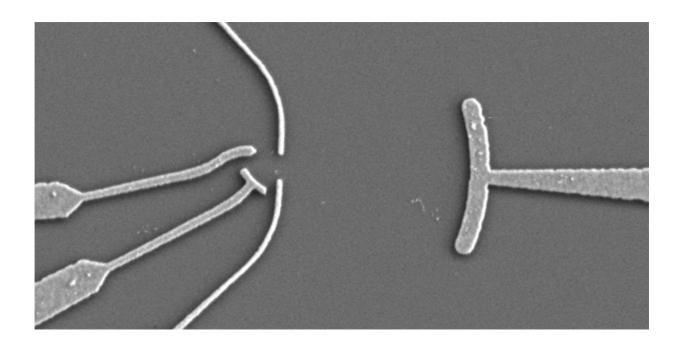
Electron microscope image of the ETH Zurich experiment. Between the quantum dot (left) and the curved electrode (right) electronic standing waves arise, which interact with the electrons of the quantum dot. Credit: Rössler C et al. Physical Review Letters 2015
