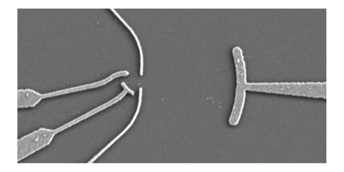
Electron microscope image of the ETH Zurich experiment. Between the quantum dot (left) and the curved electrode (right) electronic standing waves arise, which interact with the electrons of the quantum dot. Credit: Rössler C et al. Physical Review Letters 2015
