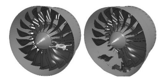
Researchers at the Virginia Tech College of Engineering have created computer animes of what would happen if a drone were pulled into a commercial airliner's turbo fan engine block.
