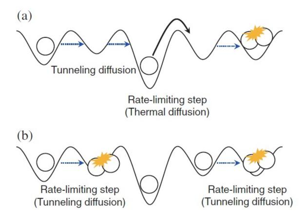
Illustration of surface diffusion of atoms, with the blue arrows showing quantumtunneling diffusion (through classical barriers) and the black arrow showing thermal hopping. The figure shows how the diffusion mechanisms differ for (a) low atomic flux (dominated by thermal hopping) and (b) high atomic flux (dominated by quantum tunneling). Credit: Kuwahata, et al. ©2015 American Physical Society
