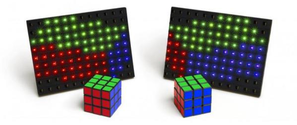
The second prototype of the 3-D display module, which sends different images to different directions, enabling glasses-free 3-D. Credit: TriLite
