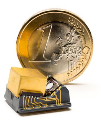
The basic element of future large-scale displays: A Trixel with a movable mirror. Credit: TriLite
