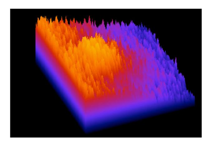
This 3-D contour map of the positron signal for one of the laser shots shows the positron signal strength relative to the pixel-level background noise in the detector. Credit: E. Liang/Rice University
