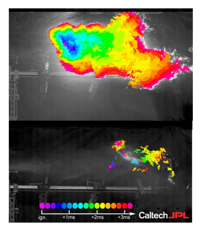
The progress of the flame after ignition in a post-impact mist of Jet-A fuel treated with prior ultra-long polymers (upper) and the Caltech polymer (lower) after the samples have passed through a fuel pump 50 times. The efficacy of prior polymers is lost, and a large, hot fireball ensues. The Caltech polymer
