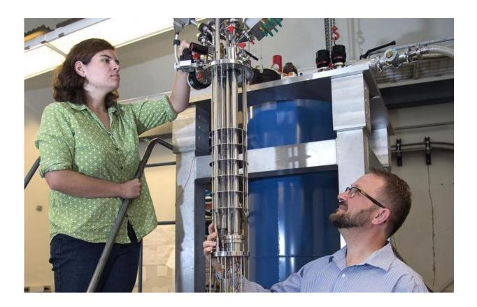
Purdue University professor Gábor Csáthy and graduate student Katherine Schreiber inspect equipment used to cool samples to near absolute zero. The equipment was used in Purdue-led research that led to the observation of an unexpected phase transition in an ultrapure material. Credit: Purdue University /Mark Simons
