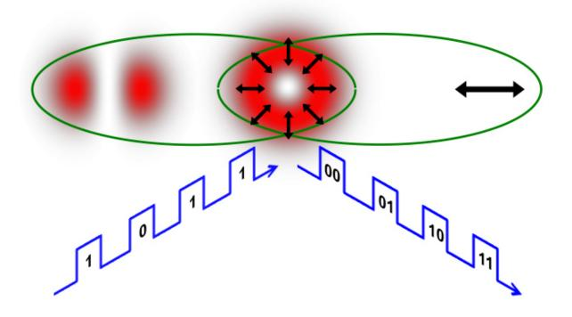
The shape and polarization of a conventional laser beam from a laser pointer mimics quantum entanglement when the laser beam has a polarization dependent shape. This can be used to encode twice as many bits of information as when the laser beam is "separable." Credit: Giovanni Milione
