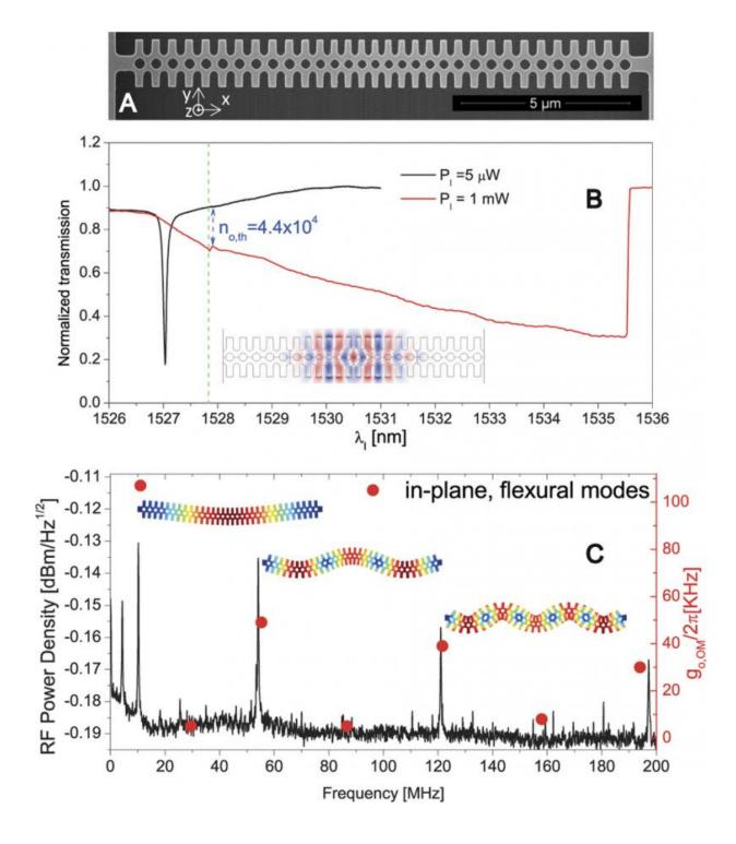
(A) SEM micrograph of the OM photonic crystal cavity. (B) Normalized transmission spectrum around the studied optical mode for input laser powers of 5  $\mu$ W and 1 mW (black and red curves respectively). The threshold for establishing the regime of self-sustained oscillation is indicated (green dashed vertical line). (C) Transduced acoustic modes up to 200 MHz. The red dots
