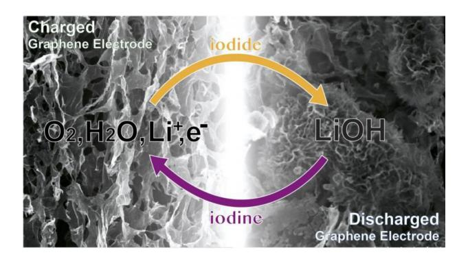
A schematic showing the formation of lithium hydroxide (LiOH) on the graphene electrode on discharging a non-aqueous lithium-oxygen battery in the presence of the redox mediator, lithium iodide, and trace water. On charging, the iodide is oxidized to iodine, which helps to remove the LiOH and reform the bare graphene electrode. Credit: Tao Liu, Gabriella Bocchetti and Clare P. Grey
