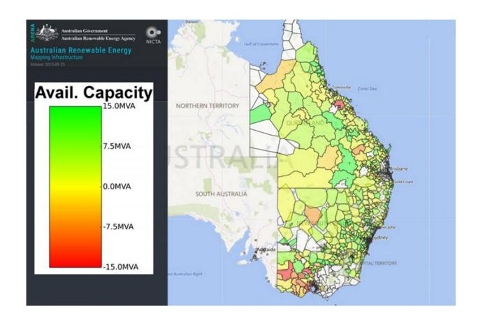
The interactive maps show where capacity-related constraints exist (orange and red) where investment will be needed to ensure reliable electricity supply. Picture supplied.
