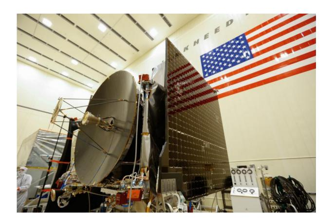
The high gain antenna and solar arrays were installed on the OSIRIS-REx spacecraft prior to it moving to environmental testing. Credit: Lockheed Martin Corporation
