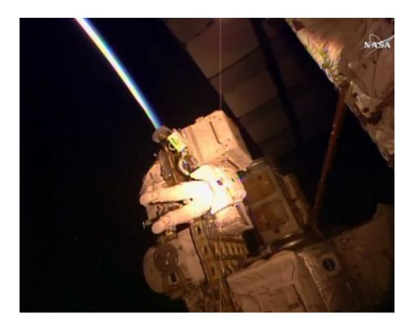
In this frame grab from NASA Television, astronaut Kjell Lindgren performs maintenance outside the International Space Station, Wednesday, Oct. 28, 2015. Lindgren and fellow astronaut Scott Kelly's to-do list included greasing the station's big robot arm, routing cables, removing insulation from an electronic switching unit and covering an antimatter and dark matter detector. (NASA via AP)
