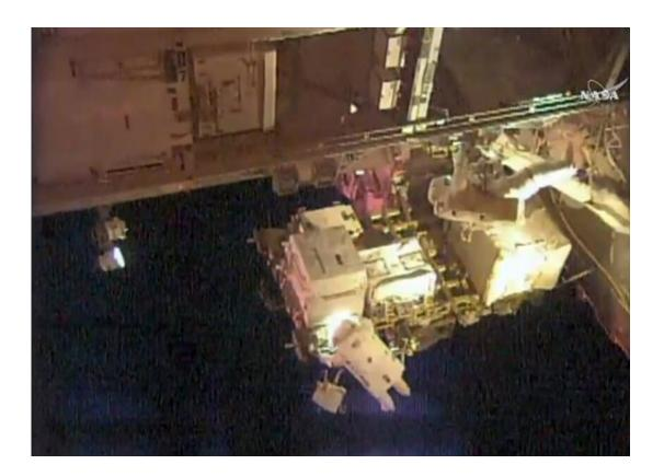
In this frame grab from NASA Television, astronauts Scott Kelly, upper right, and Kjell Lindgren, bottom, perform maintenance outside the International Space Station, Wednesday, Oct. 28, 2015. The astronauts' to-do list included greasing the station's big robot arm, routing cables, removing insulation from an electronic switching unit and covering an antimatter and dark matter detector. (NASA via AP)
