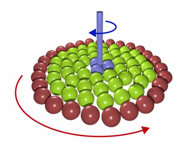
A model microscopic system to demonstrate the transmission of torque in the presence of thermal fluctuations -- necessary for the creation of a tiny 'clutch' operating at the nanoscale -- has been assembled at the University of Bristol, UK. This image shows the principle of operation of the 'nanoclutch': red spheres rotate clockwise and an opposing torque is applied to a central axle. Credit: Dr Paddy Royall, University of Bristol
