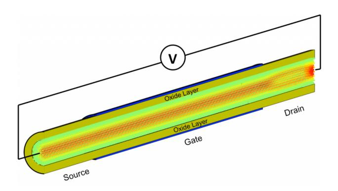
Spatial distribution of the electron current flowing through a silicon gate-allaround nanowire field-effect transistor composed of 55,488 atoms. A voltage (V) is applied to the structure. Half of the oxide-capping layer is removed to shed light on the interior of the transistor where the atoms are colored according to the current they carry: green means no current, whereas red indicates a high concentration.
