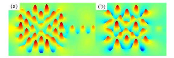
Mode field patterns for a square resonator with a side length of  $2.5 \,\mu m$  connected with a waveguide. Credit: Science China Press
