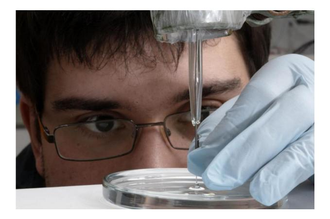
Not the complete platinum surface is catalytically active, but only some especially exposed areas, so-called active centers. Measurement of a platinum electrode with a hanging meniscus configuration. Credit: Wenzel Schuermann, Technical University of Munich
