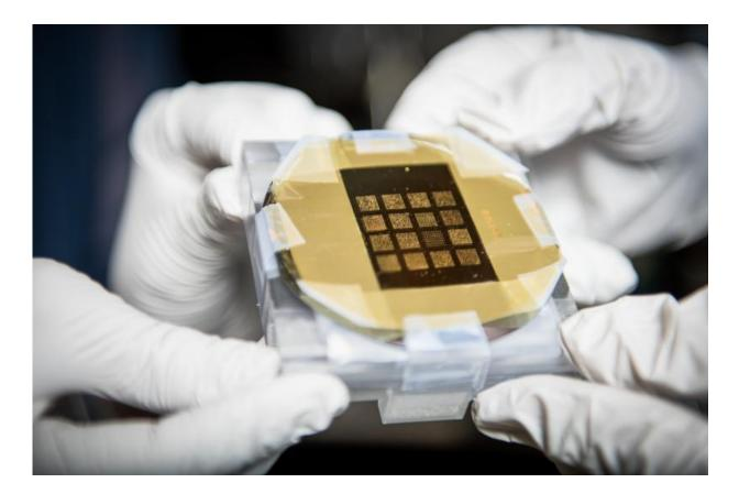
An emerging class of materials, metamaterials consist of specially designed metal patterns on the substrate, like silicon, whose size, geometry and orientation can be selected to allow for exotic optical properties The device fabricated by the UA researchers can be on both flexible substrate and silicon.
