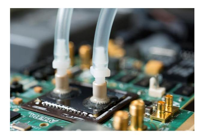
Liquid ports carry cooling water to specially designed passages etched into the backs of FPGA devices to provide more effective cooling. The liquid cooling provides a significant advantage in computing throughput. Credit: Rob Felt, Georgia Tech
