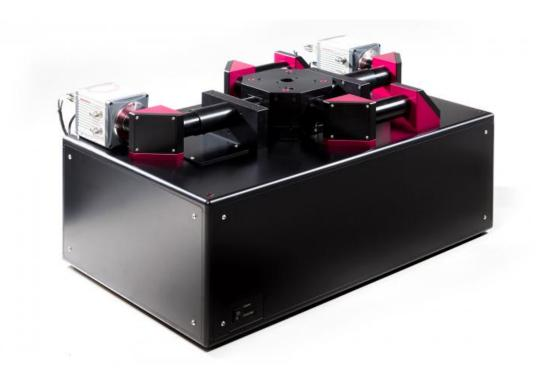
The MuVi-SPIM microscope enables scientists to observe living cells in three dimensions, for extended periods of time. Credit: Luxendo
