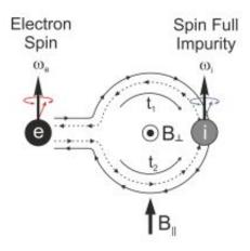
Researchers at Chalmers University of Technology shows that applying a moderate in-plane magnetic field increases spin lifetime of electrons in graphene. The results of this work have profound implications for graphene's use as post-CMOS platform in spintronics, and make an important contribution to the understanding of physics of 2D materials. The findings have recently been published in the prestigious journal *Physical Review Letters*.
