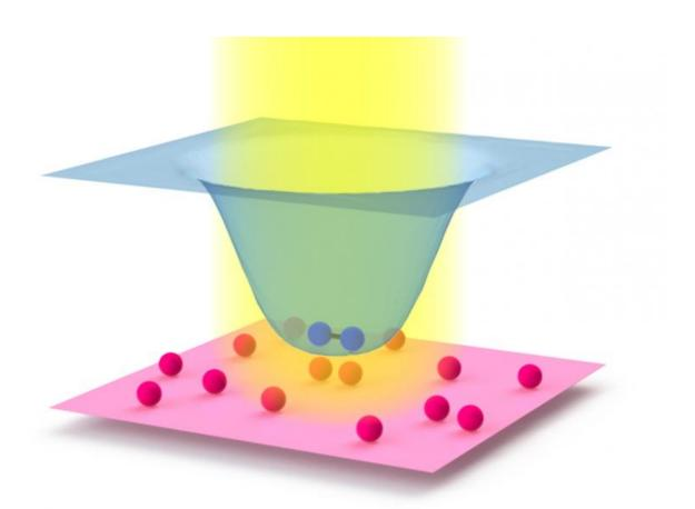
This image shows how a laser (yellow) can affect collisions between atoms (red spheres). The blue spheres depict a molecule. The laser leaves the energy of single atoms unaffected, as represented by the red surface. But the laser lowers the energy of the molecules, leading to the cup-shape of the blue surface. The stronger the laser, the more the two atoms attract each other if they collide inside the laser beam. Credit: Chin Group/University of Chicago
