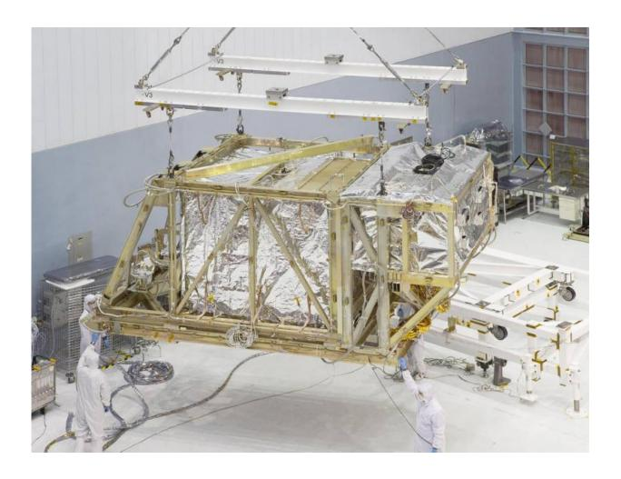
The James Webb Space Telescope team lifts the Integrated Science Instrument Module (ISIM) structure by crane as it leaves the Goddard clean room for the thermal vacuum chamber. Credit: NASA/Chris Gunn
