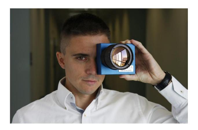
A spin-off of the Universidad Carlos III de Madrid (UC3M), Sensia Solutions, has developed a new low-cost infrared camera that makes it possible to quickly and efficiently detect gas leaks that can occur in different industrial facilities. Credit: uc3m
