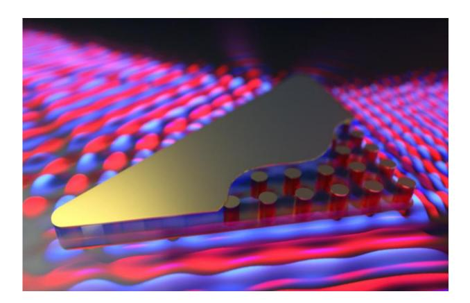
In this zero-index material -- made of silicon pillar arrays embedded in a polymer matrix and clad in gold film -- there is no phase advance. Instead zero-index material creates a constant phase, stretching out in infinitely long wavelengths. Credit: Peter Allen, Harvard SEAS
