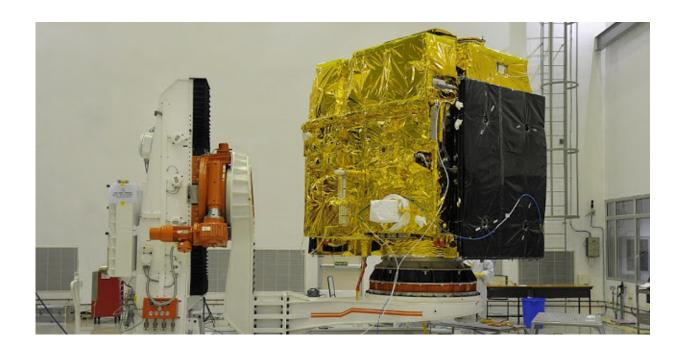
Astrosat during a pre-launch test in a clean room. Credit: ISRO
