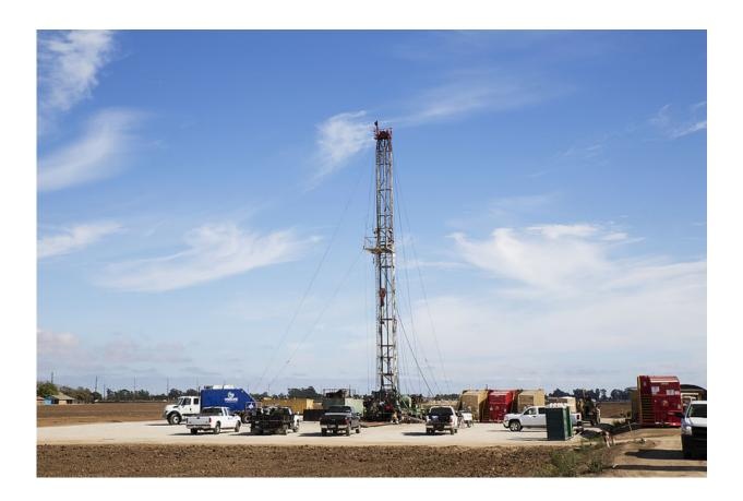
A fracking well injects large volumes of water, chemicals and sand to fracture rock. Credit: 128012869@N08/flickr, CC BY-NC-ND
