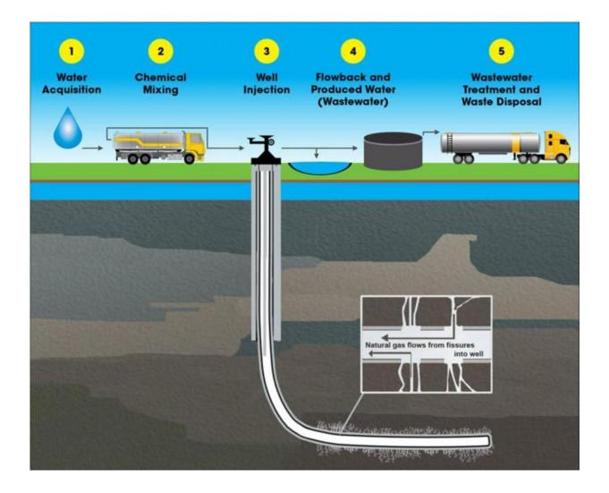
Wastewater from hydraulic fractured wells is collected and disposed of in containment pools or, for permanent disposal, in injection wells. Credit: EPA
