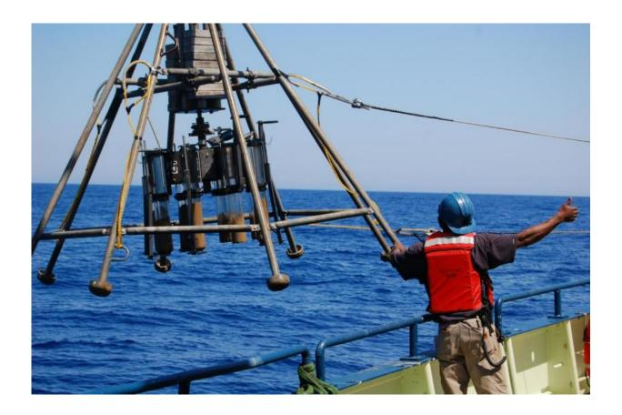
This shows a sediment coring device that simultaneously takes eight short 1-foot cores of the sediment surface from the seafloor. These short cores are useful because they capture the uppermost, youngest sediments, thus allowing scientists to measure sediment accumulated during the past several thousand years. Credit: Peter deMenocal
