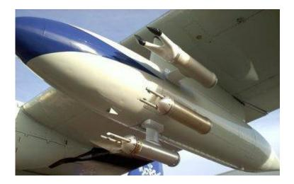
The HOLODEC instrument, or Holographic Detector for Clouds, is mounted to and transported via a C-130 aircraft. Credit: NCAR
