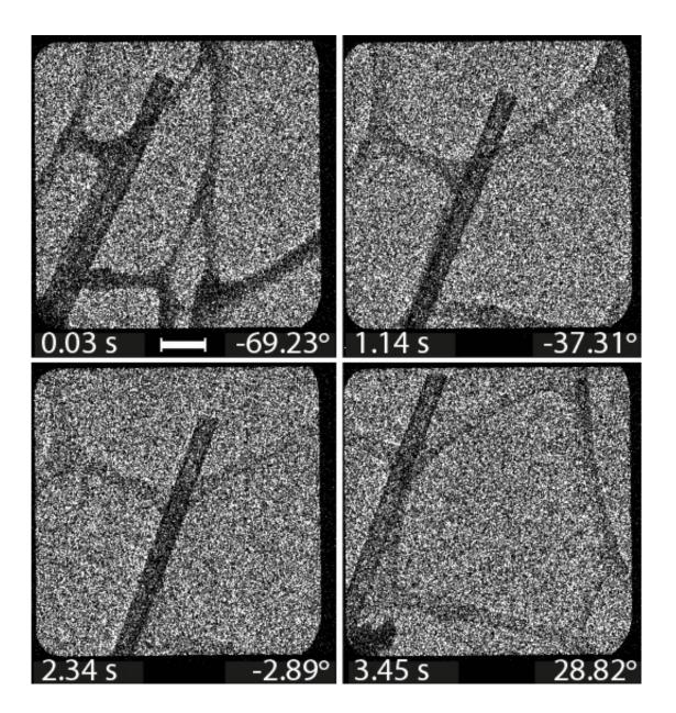
The image series serves as a data basis for the reconstruction of the 3D electron tomogram. Credit: Migunov, V. et al. Sci. Rep. 5, 14516, 2015
