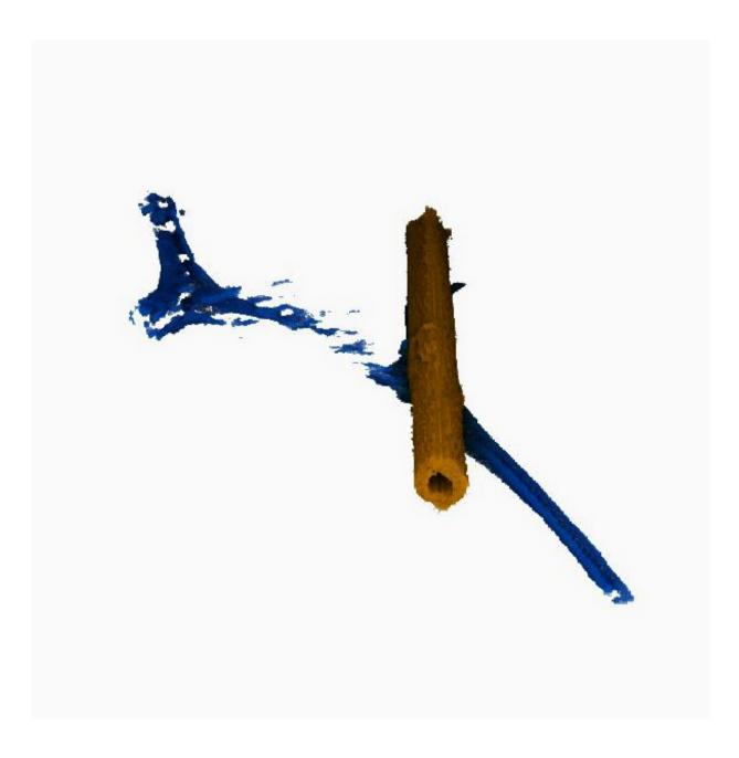
3D electron tomogram of a nanotube (orange) and the underlying amorphous C
