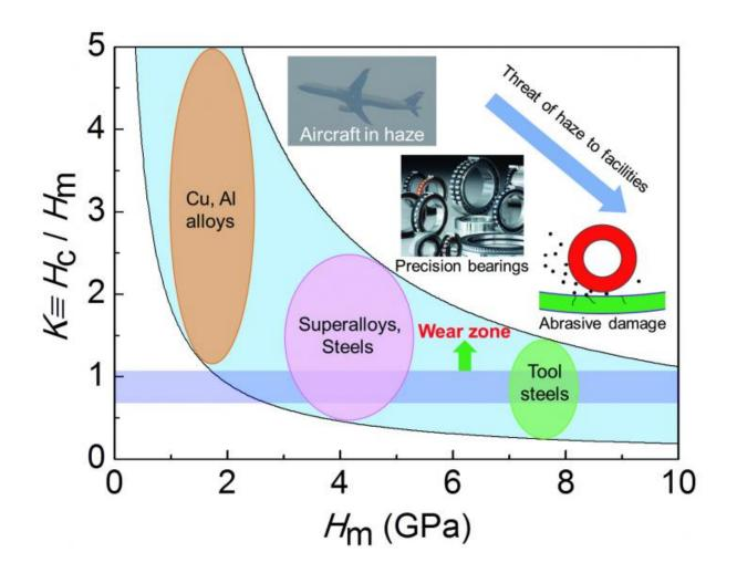
Critical criterion for haze particles to generate abrasive damage to alloys. Credit: ©Science China Press
