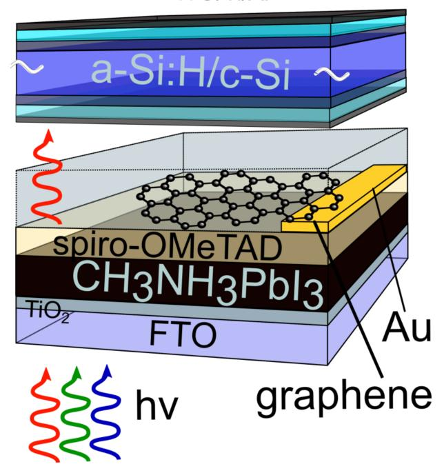
The perovskite film (black, 200-300 nm) is covered by Spiro.OMeTAD, Graphene with gold contact at one edge, a glass substrate and an amorphous/crystalline silicon solar cell. Credit: F. Lang / HZB
