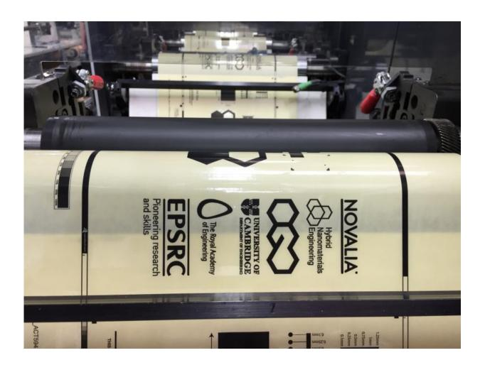
Graphene ink being roll-to-roll printed. Credit: Tawfique Hasan
