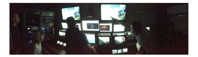
Pilots and scientists inside the control van of the remotely operated underwater vehicle view the underwater scene in real time, collecting samples, images, and oceanographic data. Credit: Peter Auster
